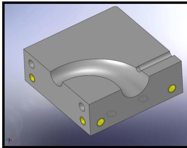
The picture above shows the designed 3D geometry. The shape is a 90° bent cone, which tapers along the curve. The G-code programming solution for that geometry is limited. With VisualMILL, the machining operations for roughing and finishing were done. The desired traversing path and other safety margins could have been always changed to get the optimal tool paths.
