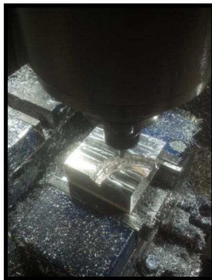
The picture above shows the DMU 35, milling the cavity only with coordinates from VisualMILL. The duration of processing was approximately 20 minutes.
