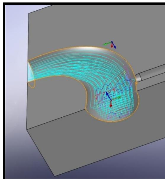
The picture above shows VisualMILL's tool path for the inner contour.
