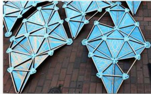
Rhino Grasshopper was then used to modify every curve so that it started at the surface and plunged a maximum of 1/8 of an inch into the surface and then gradually come back out in a feathering pattern on each end. We then showed them how easy it was to use RhinoCAM to generate engraving toolpaths and the g-code necessary to cut each of their unique panels.
