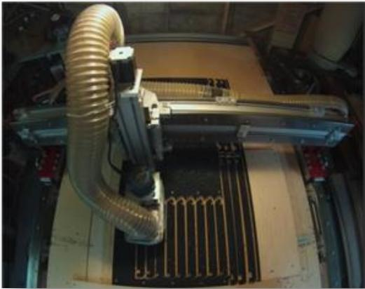
The important thing in this project according to Scott was RhinoCAM's ability to automatically create bridge points to hold all of these pieces in place within each 4x8 sheet. No vacuum table was used. The nesting of the parts and the bridge points designed in RhinoCAM allowed each part to be held in place just long enough until the next piece is cut, thus removing the bridge points from the previous cut.
