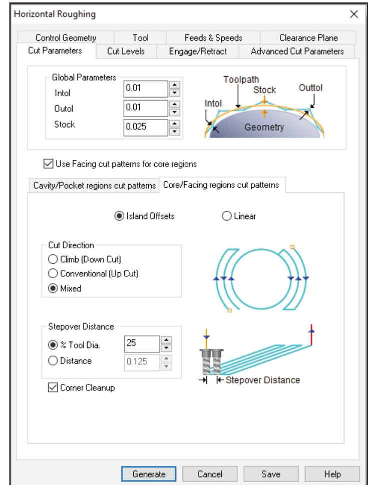
The VisualMILL Horizontal Roughing operation dialog is displayed, showing the Core/Facing selections of the Cut Parameters tab for the ukulele neck.
