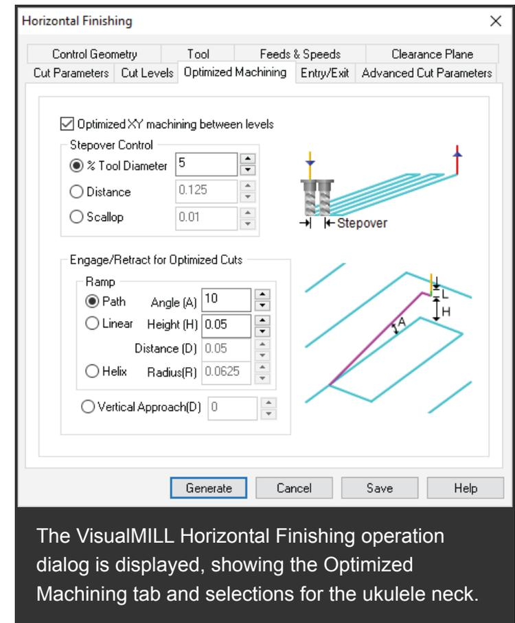
Optimized Machining automatically recognizes these flat areas and inserts projection toolpaths, similar to 3 Axis Projection Pocketing to clean out unmachined areas. This is a highly effective way of maintaining a uniform scallop height on the part. You have Stepover Control of the spacing of these optimized toolpaths as well as Engage/Retract for Optimized Cuts as shown in the dialog above.
