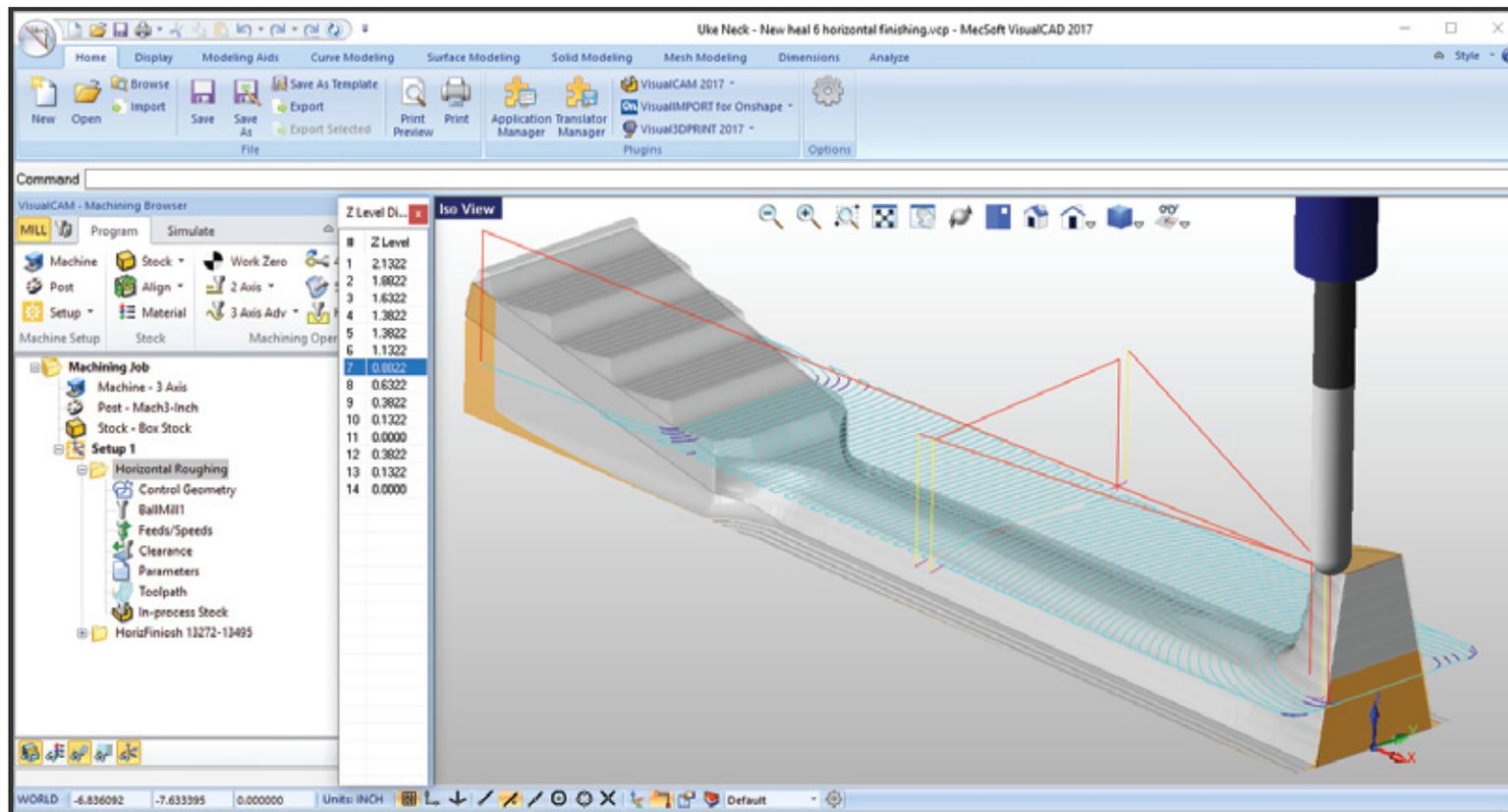
In VisualMILL 3 Axis Horizontal Roughing you can view each Cut Level independently using the Z Level Display dialog (shown here to the right of the VisualMILL Machining Browser).
