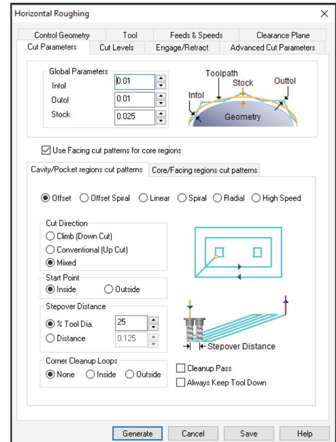
The VisualMILL Horizontal Roughing operation dialog is displayed, showing the Cavity/Pocket selections of the Cut Parameters tab for the ukulele neck.
