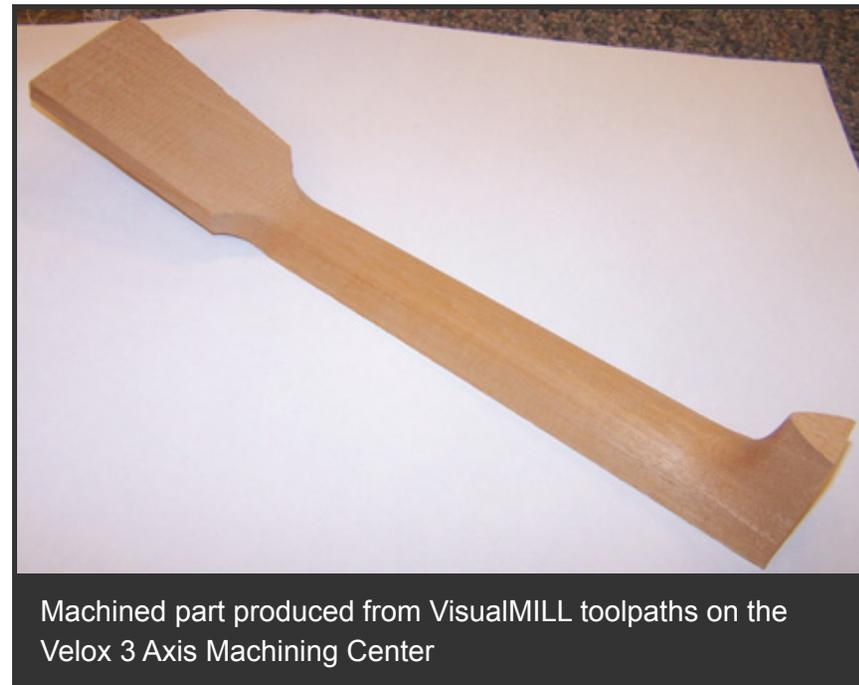
3 Axis machining is needed for this part due to the drafted walls and curvature design required. Tony and his team uses 3 Axis Horizontal Roughing for bulk material removal followed by 3 Axis Horizontal Finishing. The sections below provide a glimpse into these machining strategies and the parameters used for this part.
