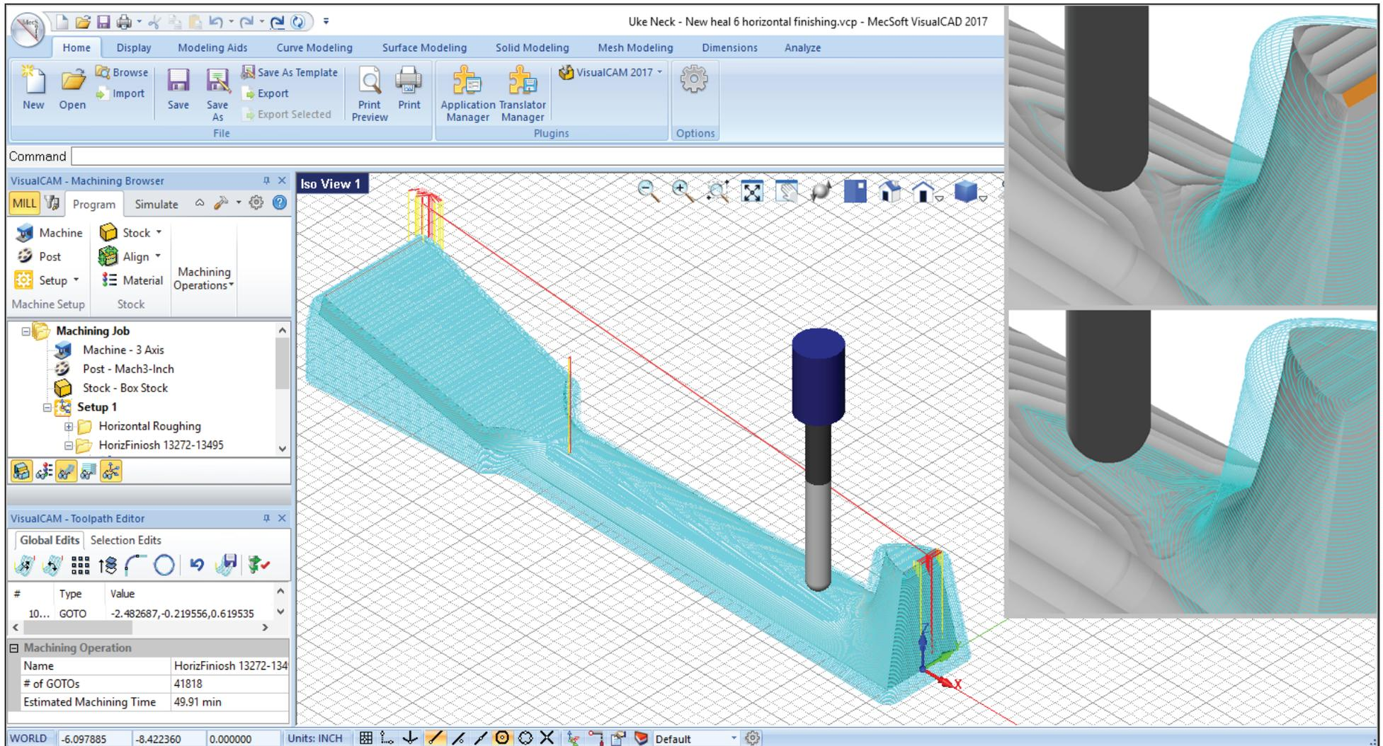
In the main image, we see the entire 3 Axis Horizontal Finishing toolpath displayed in VisualMILL. (Inset Bottom Right) With Optimized Machining enabled, the step over distance in the flatter areas matches the Z step down distance in the vertical areas, resulting in a constant scallop height and finer surface finish.
