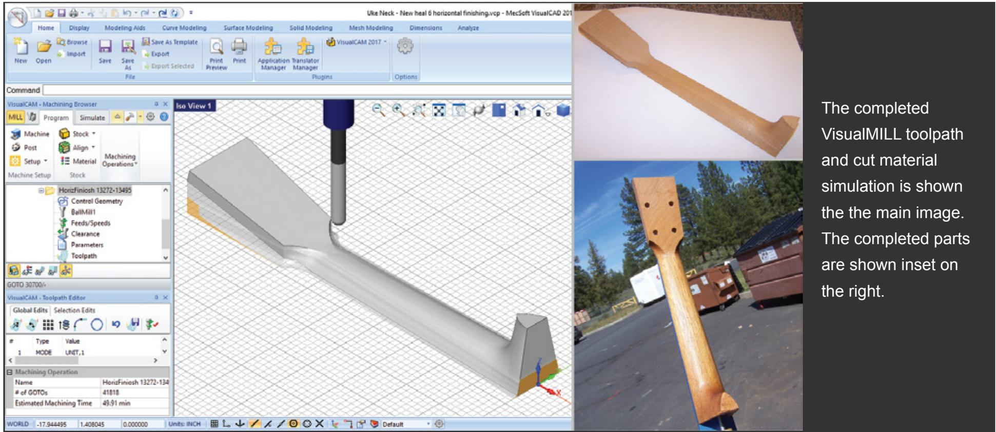
The completed VisualMILL toolpath and cut material simulation is shown in the main image. The completed parts are shown inset on the right.
