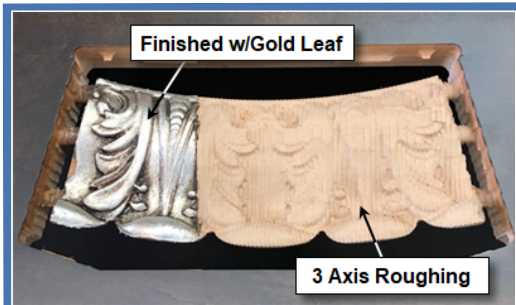
Example in-process stock of curved Acanthus Crown Molding section.
