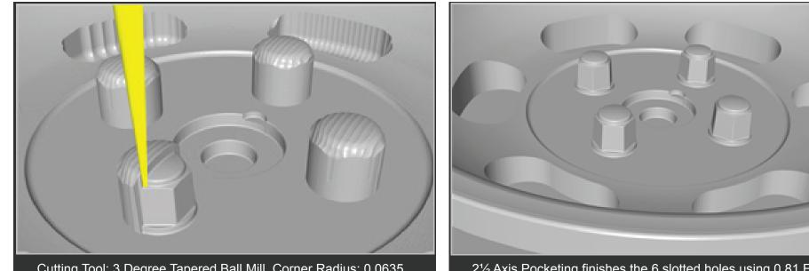
Cutting Tool: 3 Degree Tapered Ball Mill, Corner Radius: 0.0635 Flat Dia.: 0.00017, Step over: 5%
