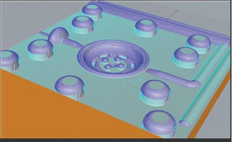
Parallel Finishing using a 1.02 dia Ball Mill, 25% step over leaving 0.3 of stock.
