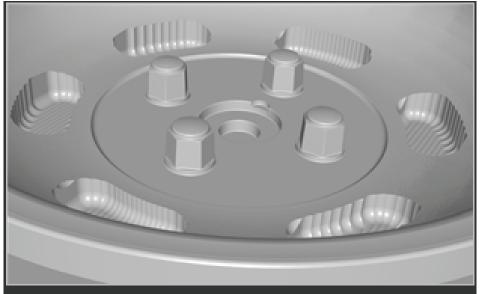
After pocketing the center cap, Jim uses a Tapered Ball Mill and Parallel Finishing to complete the 4 lug nuts.
