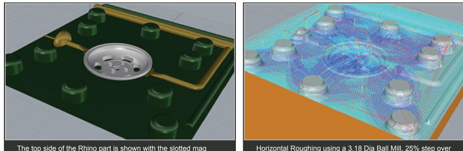
The top side of the Rhino part is shown with the slotted mag wheel in the center. The locator pins are in green and the sprue lines are in gold.
