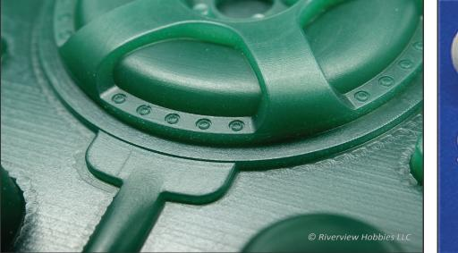
The Porsche 934 wheel kit wax mold machined from RhinoCAM toolpaths
