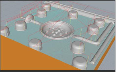
Parallel Finishing using a 0.81 dia End Mill, 50% step over leaving 0 stock. This toolpath is contained to the perimeter of the flat parting plane areas only.
