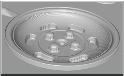
Here we see the results of a 3 Axis Pencil Trace (0.81 Dia. Flat End Mill),  $2\frac{1}{2}$  Pocketing and a 3 Axis Horizontal Finishing (0.51 Ball Mill), all on the outer rim.
