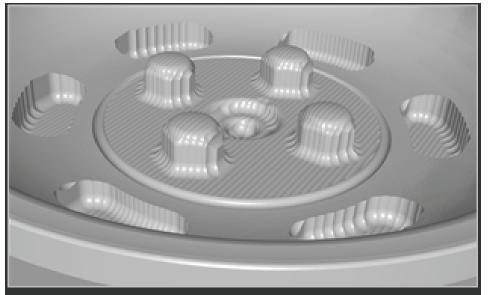
After zooming in, we see the results of another Horizontal Finishing toolpath, this time on the outer hub. To really appreciate the control and accuracy of RhinoCAM, have a look at the next two images.
