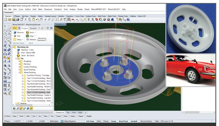
(Main Image) Shown modeled in Rhino, is a prototype mold cavity of the Riverview Hobbies RVH121001 Slotted Mag Wheel Kit for the 1/12 Tamiya Datsun 240ZG model kit. On the left we see the RhinoCAM MILL Machining Browser listing toolpaths for the indexed 4 Axis machining job. (Top Right) A production component is shown. (Bottom Right) The 1/12 Tamiya Datsun 240ZG model kit is shown complete with the Riverview Hobbies RVH121001 Slotted Mag Wheel Kit.
