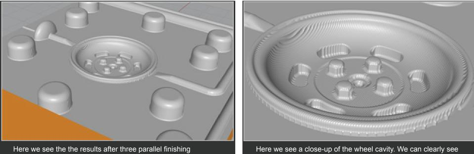
operations contained to the locator pins, bar and sprue. A 0.81 Ball Mill is used with a stepover of 10% (that's 0.003" step over!).
