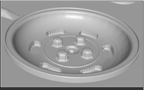
After another Parallel Finishing toolpath, this time between the outer rim and the center cap using a 0.51 Dia. Ball Mill and a step over of 0.01 (that's 0.0004")
