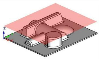
**Display of Clearance Plane for Milling operations**
