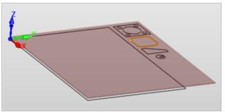
Display of Clearance Plane for Milling operations
