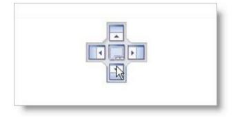
For example: Selecting the button on the widget with arrow pointing downwards on and releasing the left mouse button docks the selected browser below the specified browser.
