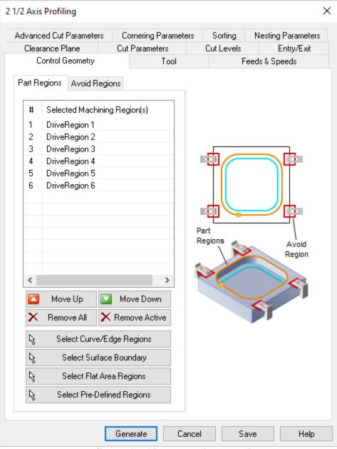
Profile Operation Dialog Box: Control Geometry tab
