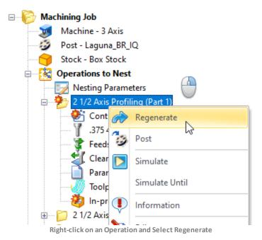
The toolpath is now generated with the modified settings. Notice that the In-process Stock is still flagged. This alerts you that it has not been simulated yet.
