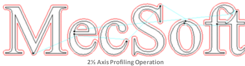
2½ Axis Profiling Operation
