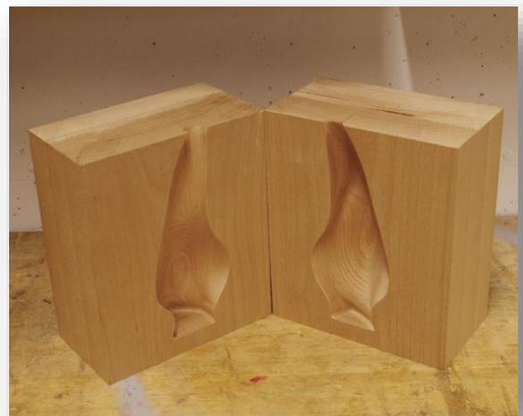
The mold cavities are completed and ready for glassblowing.
