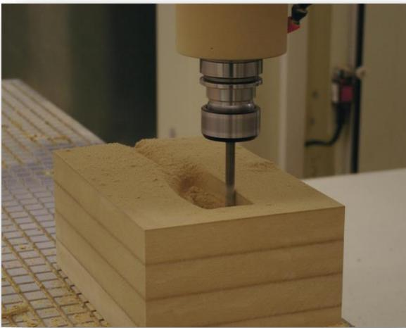
Machining the mold cavities for the carafes.
