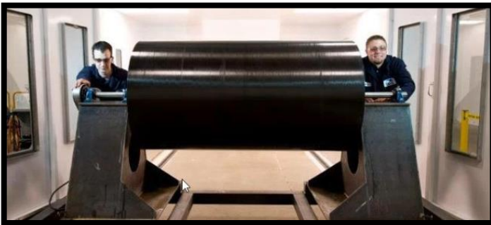
Figure 2 - Flywheel from Beacon Power, LLC in Tyngsboro, MA and the Stephentown, New York facility
