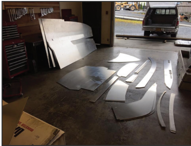
Figure 6 – Aluminum components for the full-size 10-foot aluminum tram cut from RhinoCAM toolpaths by students in the Wrangell Public High School's Marine Fabrication class.
