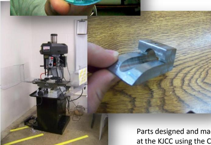
The type of toolpaths created in the Computer Aided Drafting class, taught by Matt Dunning, lent itself more to 3 Axis and 4 Axis machining. Small machine components made of brass or aluminum was what was usually machined there. The challenges in machining here were more related to part fixturing, since typically the parts were multi-sided. With VisualMILL's 4<sup>th</sup> axis machining capabilities this is easily accomplished.
