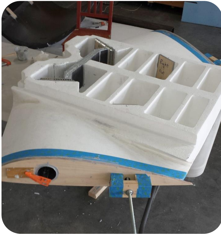
The wingbox foam core with wood bulkheads and titanium tubing spars
