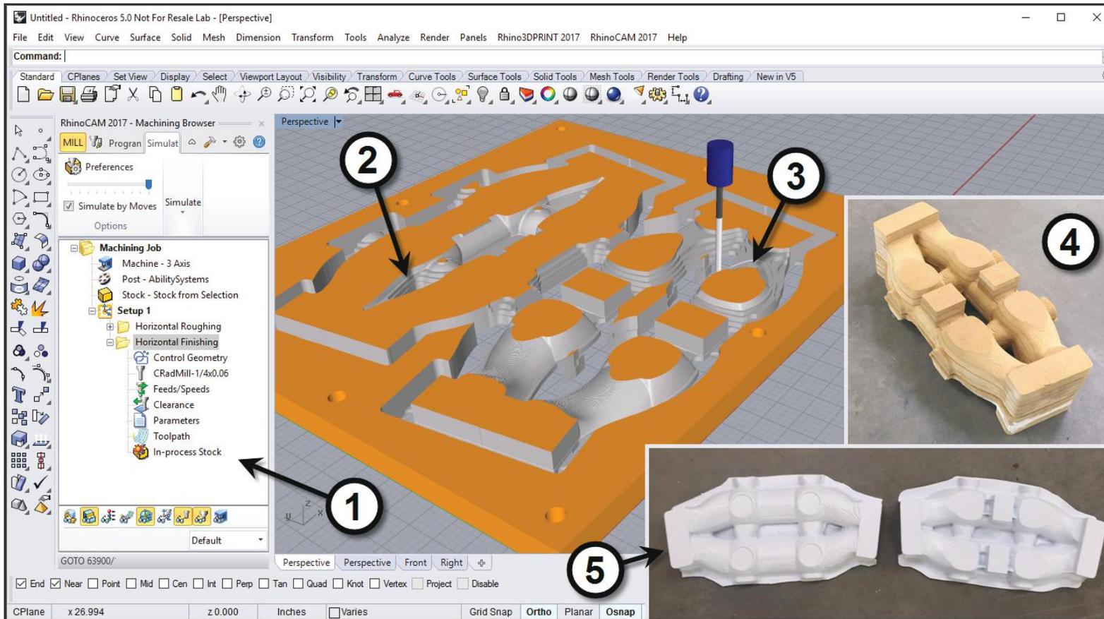
Toolpaths for a section of the Green Wall pod are displayed in RhinoCAM along with the pod core and resulting vacuum formed core halves. Refer to the more complete description in the text below.
