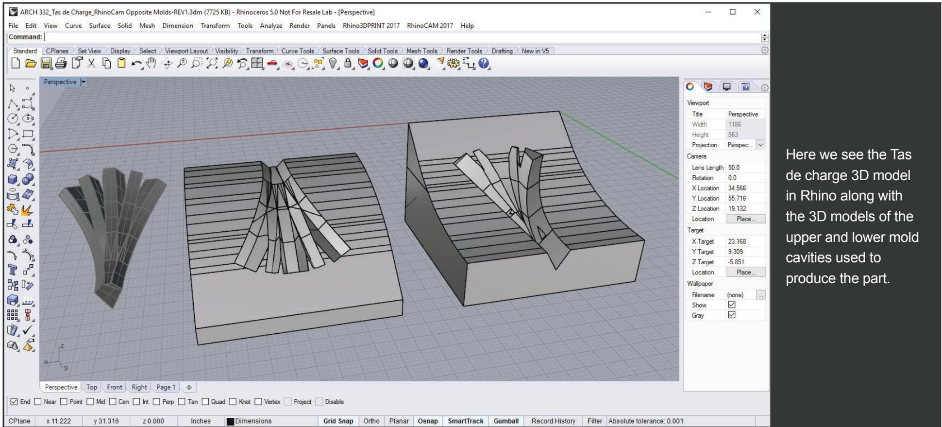
Here we see the Tas de charge 3D model in Rhino along with the 3D models of the upper and lower mold cavities used to produce the part.
