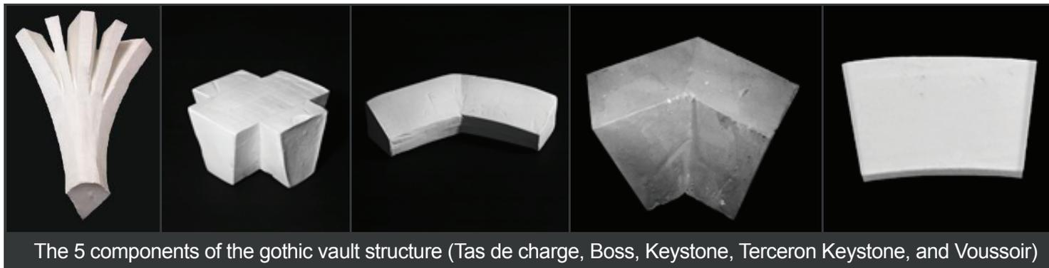
Here are the 5 components of the vault structure from left to right ([Tas de charge](#), [Boss](#), [Keystone](#), [Terceron Keystone](#), and [Voussoir](#)). While this is a group project, each student has access to the actual Rhino parts and assembly for 3D modeling and RhinoCAM for programming toolpaths on the school’s 3 Axis Techno CNC machining center. Since the Tas de charge is the most complicated piece, we have selected it for further discussion below.
